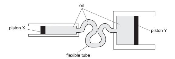
When the driver presses on the brake pedal, a force is exerted on piston X. The pressure produced in the oil by this force is transmitted through the oil so that it causes a force to act on piston Y. This presses the brakes against the moving parts.
