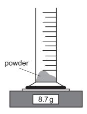
Liquid is poured into the cylinder to cover the powder completely. The powder does not dissolve. The reading on the measuring cylinder and the reading on the balance are recorded.
